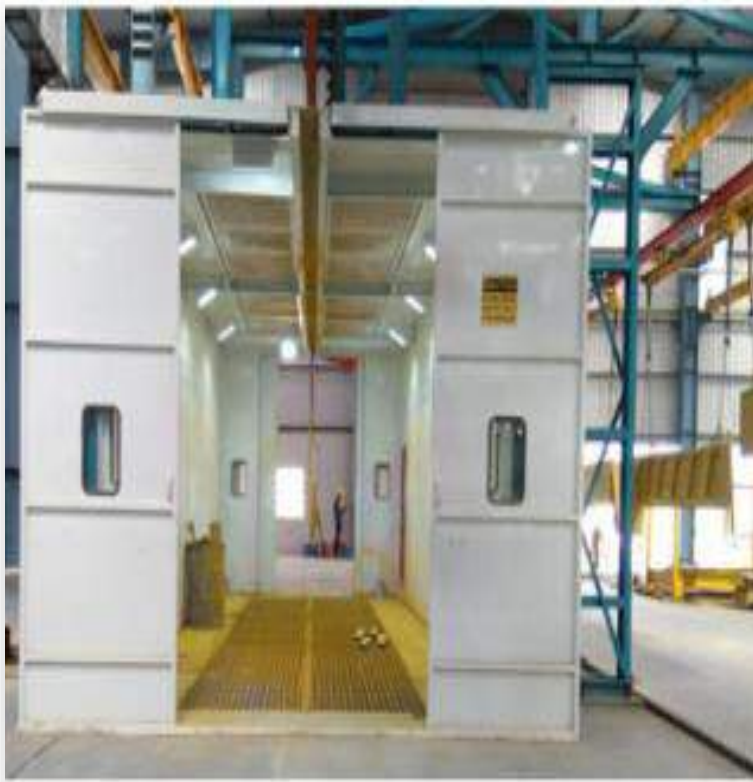
Dry filter technology Paint booth
